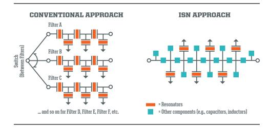
The conventional approach to RF filter design relies on a single component – resonators. Only one topology (or configuration) is possible. In contrast, ISN uses additional components, including capacitors and inductors, which enables the company to develop an infinite number of topologies. It can then select the optimal design for each specific band.
